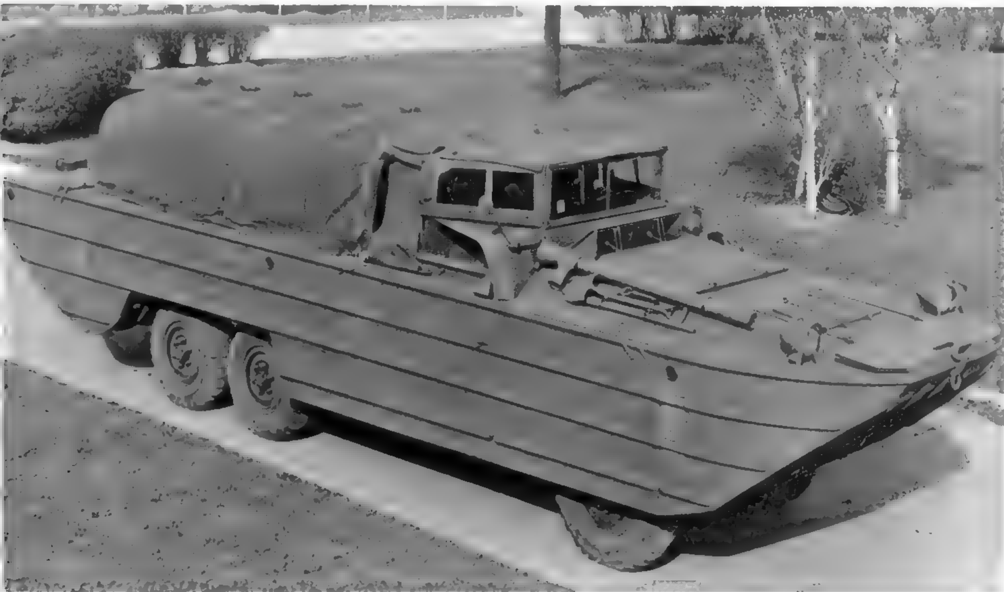
Shown here is one of the earlier DUKWs. Notice that the windshield is mounted vertically. In June 1943 the design was changed to have a sloping windshield. The rearmost reflector was moved in February 1943 to prevent it from being obscured by rope fenders. (U.S. Army photo)
